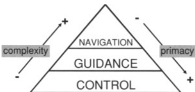
FIGURE 13.2. The three hierarchical levels of the driving task (according to Alexander and Lunenfeld, 1986).
